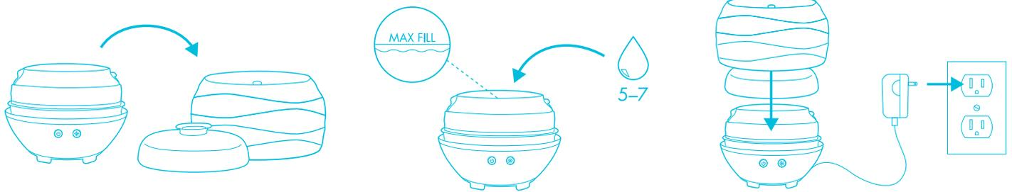
1. Remove the outer cover from the base. Next, remove the inner cover.
