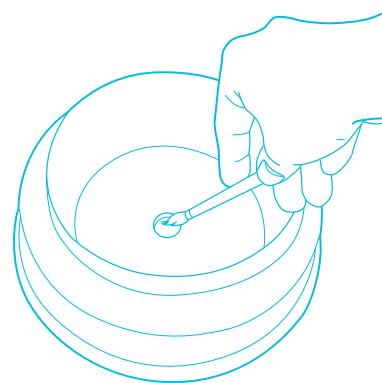
For the most thorough clean, pour a 50/50 mixture of vinegar and water into the reservoir, and let it soak for 5 minutes. Brush reservoir walls, base, and ultrasonic membrane clean with a soft-bristle brush (not included) and rinse. NEVER touch the ultrasonic membrane with your fingers, as the natural oils in skin can damage the membrane.
