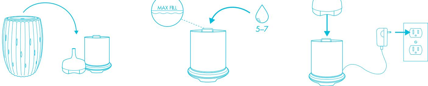
1. Remove the outer cover from the base. Next, remove the inner cover.
